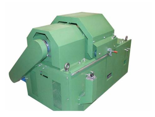
TCCM provides the latest in Machine Design Technology using 3D Modeling CAD programs for the production of small and large diameter Babbitt Bearing shells. The Model HCBLM-16 can produce single piece or split shell bearings in sizes ranging from 3" - 12" (75-305 mm) Bearing shell outside diameter, up to 12" (305 mm) long using the Centrifugal Casting process. Low profile and heavy duty enough to handle the load. No special foundation or utilities required.
