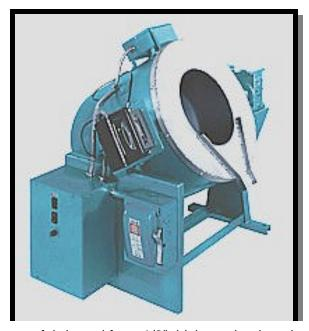
**Babbitt** Melting Pots are fabricated from 1/2" thick steel or heavier using welded steel construction. Heating elements are mounted to the inner casing walls with grooved porcelain retainers. The elements radiate uniform heat directly to the pot outer surface walls. This quickly and effectively transfers the heat to the material you are melting. This method prevents pot stresses and ho spotting that tends to shorten pot life.
