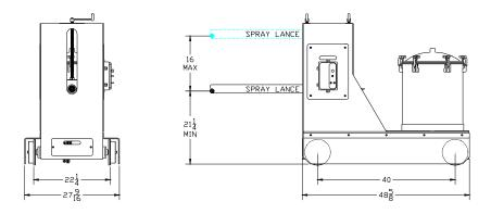
The Model ASA Spray car assembly has a 16" [406 mm] height adjustment range to accommodate a variety of permanent steel mold center-lines.
