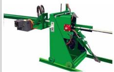
Combination mold spray and casting extractor, adjustable hydraulic traverse with pneumatic clamping for casting extraction.
