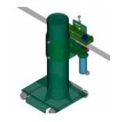
Floor mounted static unit with traversing spray lance. Adjustable variable speed lance control.
