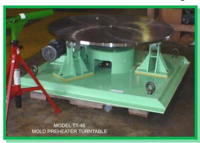
Minimize down time and increase production by preheating permanent steel molds. This "Off site" turntable can help eliminate thermal shock to the molds and prepare them for subsequent spraying of your centrifugal mold wash. No special foundation is required and with a slow rotating motion, the molds can be uniformly heated.
