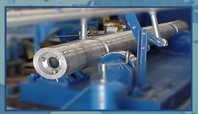
\*Casting diameter and length, with die, must not exceed total spin load capacity of Model K machine.
